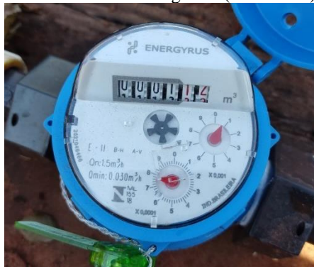
Figure 23 – Hydrometer at the beginning of manual irrigation (1120 liters).
