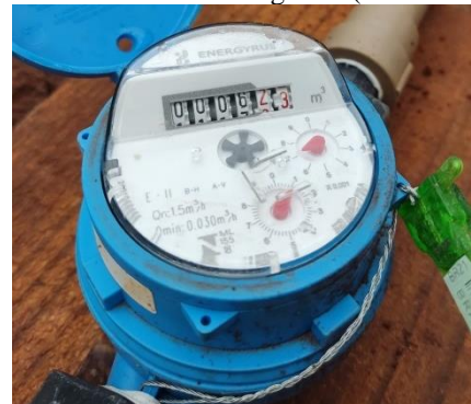
Figure 24 – Hydrometer at the end of manual irrigation (6230 liters).
