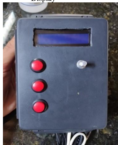
Figure 1 - Buttons, Encoder and LCD Display
