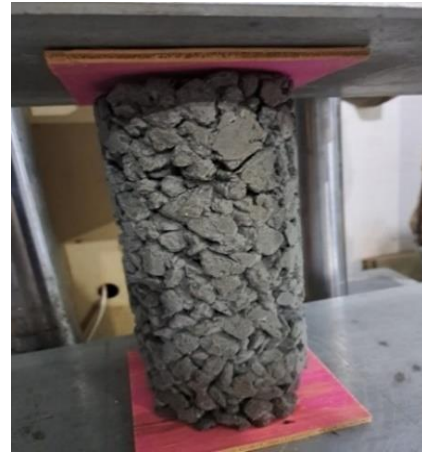
(b) Pervious Concrete
